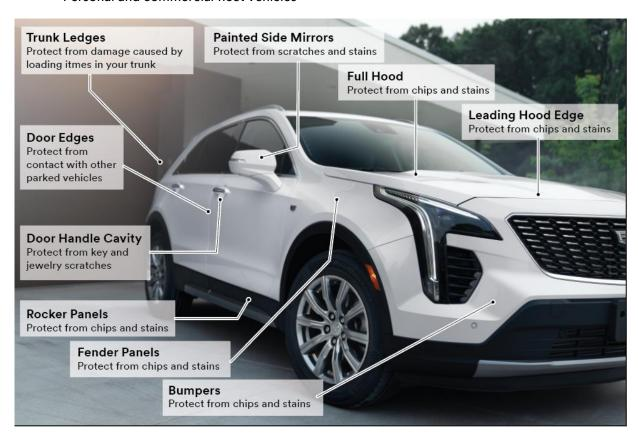
Applications shown above indicate typical areas of placement on personal vehicles. Actual film placement will vary according to the needs of the customer.
